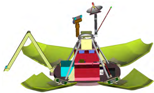
(A) Lander design provides access and fields of view for all instruments meeting Lander science requirements.
