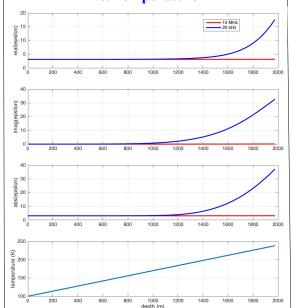
Real and imaginary parts (upper two panels) and magnitude (third panel) of the complex relative permittivity of impure water ice (50 micromolar chloride concentration)<sup>5,6</sup>, versus depth, in a 2 km-thick brittle lid model with a linear temperature gradient (lower panel). Note strong dielectric variation at 20 kHz, vs. little variation at typical radar sounding frequencies (e.g., 10 MHz).
