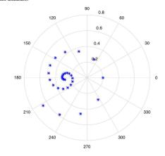
Reflection coefficients as above except at 90 kHz frequency, and with depths beginning at 100~m (at magnitude near 0.65~and phase near 210~degrees) and proceeding in 100~m increments to 3000~m thickness.
