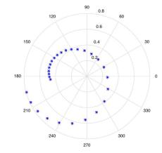
Reflection coefficients (magnitudes and phases, on a polar plot) at vertical incidence on the ice for which dielectric properties at shown at left, for 20 kHz frequency. (Computed using numerical integration of coupled first-order ordinary differential equations for electric- and magnetic-field components parallel to the ice surface, based on the method of Born and Wolfs.)
