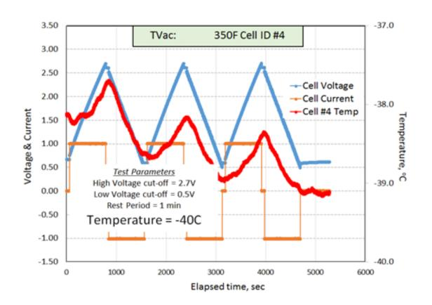
**Low ESR and linear** discharge, even at low temperatures (>350°F cells and ~5-10 m $\Omega$  at -40°C)
