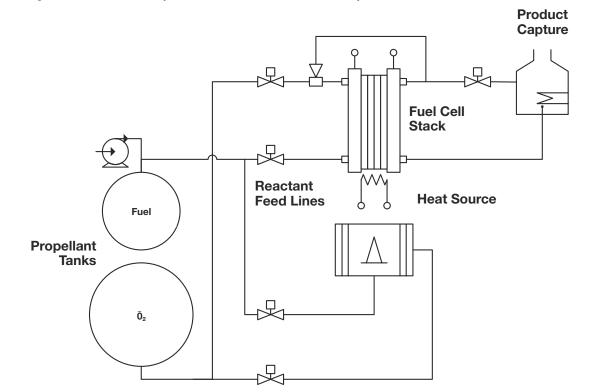
Schematic view of a fuel cell system using propellant harvesting
