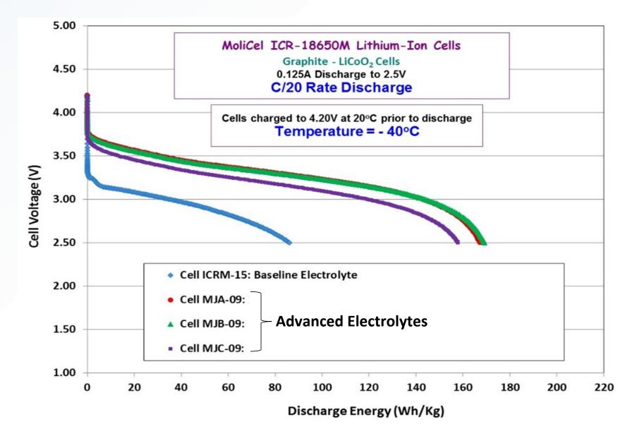
Small, cylindrical Li-ion cells with custom electrolytes outperform both COTS parts and space-rated prismatic cells, delivering a higher capacity at temperatures down to -40°C (at C/20 discharge rates)
