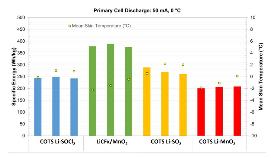
Advanced Li-CFX/MnO<sub>2</sub> cells outperform COTS/space-rated primary cells at **0°C**, delivering more capacity using the same D-cell format
