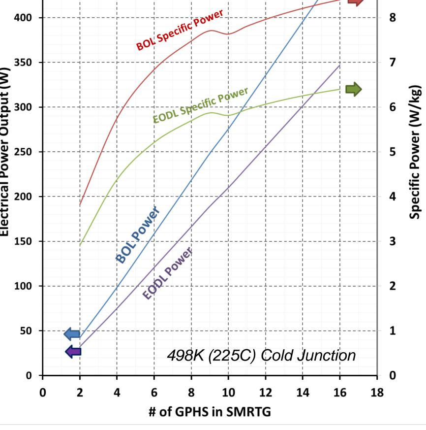
Modular System Concept Scales Over a Wide Range of Power Output and can Achieve high Specific Power
