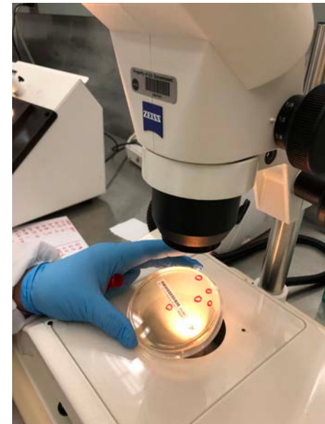
Bar coding enables reliable tracking of bioburden data
