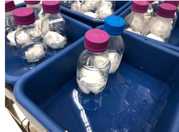
Quenching shocked samples in ice bath
