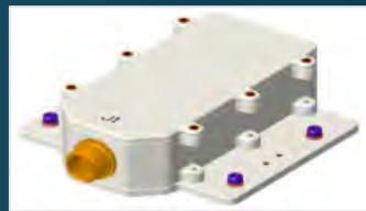
LETS Detect GCRs and SEP precursor particles
