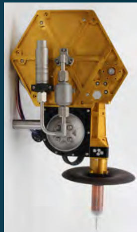
LISTER Investigate the Moon's thermal properties at depth
