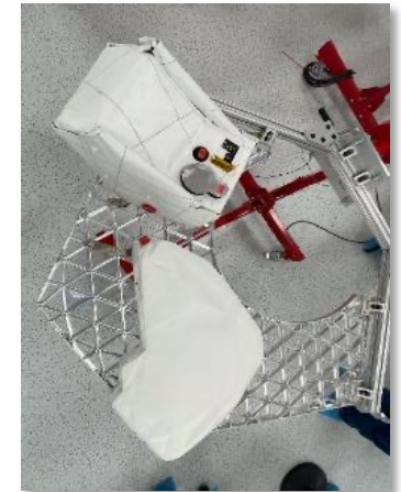
NASA payloads NIRVSS and NSS integrated onto Astrobotic's Peregrine Mission-1 lander
