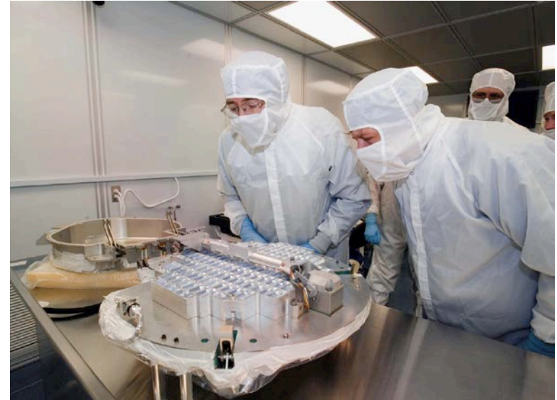
Stardust (Comet Wild 2) Samples: Returned in 2006; thousands of cometary grains in 1000 cm 2 of aerogel.
