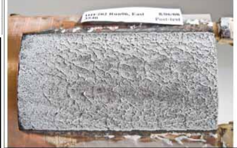
Figure 6 – Posttest Sample 3540 with 18.0-Deg Seam
