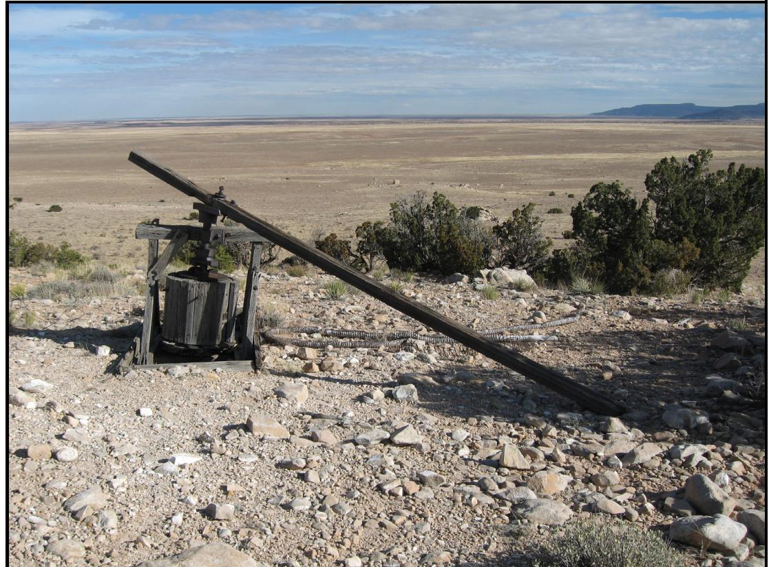
Fig. 14.14. A winch on the crater rim is a reminder of the mining exploration that once occurred at the crater. This winch was probably mule-driven and transported supplies down a slide raised above the rocky crater wall below. The winch is at the top of a large tear fault in the crater wall and rim (which is not visible in the photograph). In the middle distance, one can see blocks and mounds of Kaibab ejecta.
