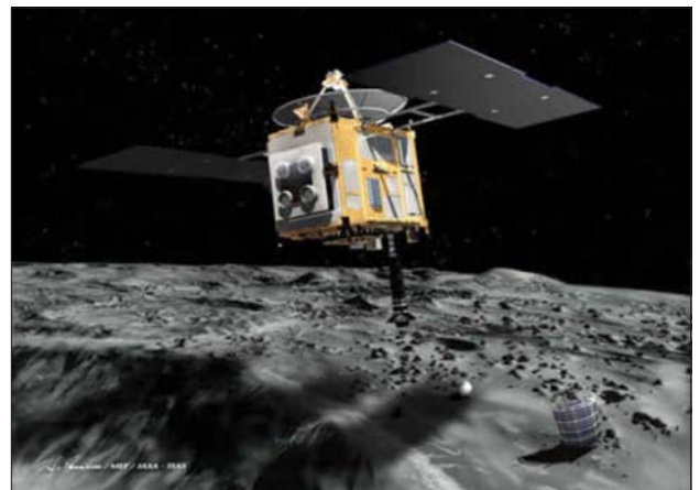
Artist's rendering showing the Hayabusa spacecraft on final approach to the surface of an asteroid. The long narrow tube extending from the base of the solar-powered spacecraft is the sampling funnel, designed to collect fragments from the surface. Credit: Japanese Aerospace Exploration Agency (JAXA).
