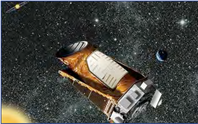
An artist's composite of the Kepler telescope. Two of Kepler's four gyroscope-like reaction wheels, which are used to precisely point the spacecraft, have failed, and NASA is ending attempts to fully recover the spacecraft.
