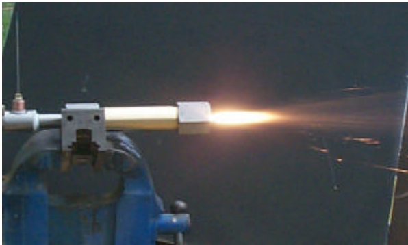
Figure 8. Test firing of hybrid rocket motor built by Rowan University students. The burning propellant is a Al/Epoxy/GOX mixture.
