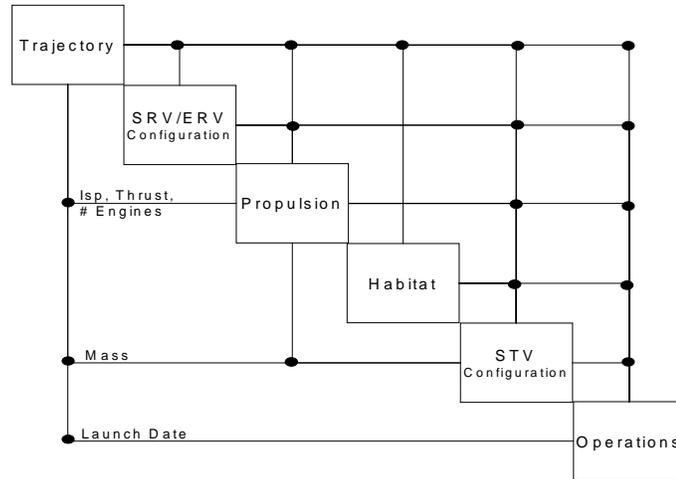
**Figure 2-1: Design structure matrix configured for fixed-point iteration.**
