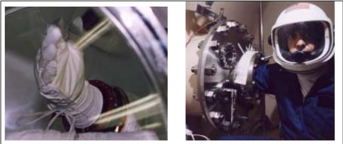
**Figure 2. Mechanical Counter Pressure Glove with EMU Lower Arm Assembly in Glovebox at -222 mm Hg Differential Pressure (left) and In Vacuum (right)**
