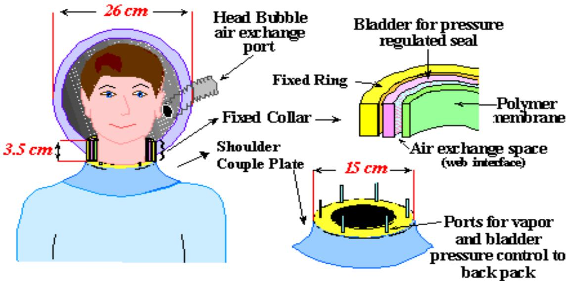
**Figure 1. Head Unit Assembly**
