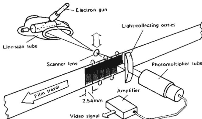
FIGURE 2.—Readout scanner.
