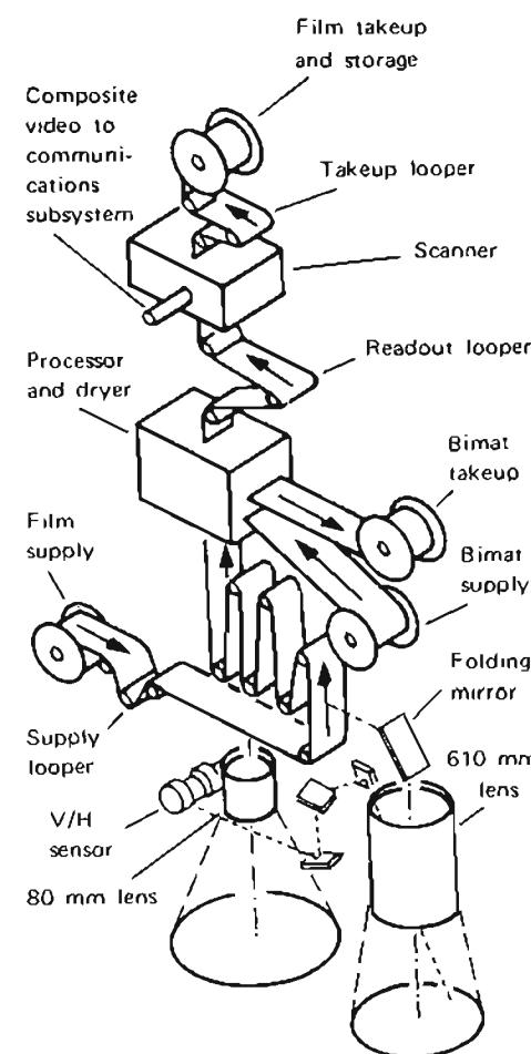
FIGURE 1.—Photographic subsystem.
