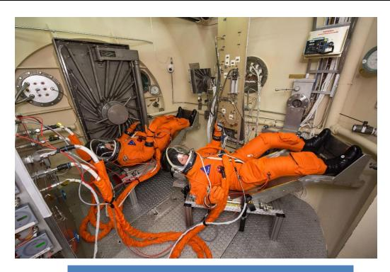
VPIST Testing is first time since Apollo that developmental pressure suits have been combined with a vehicle-level closed loop ECLSS system to provide life support while test subjects are at full vacuum.
