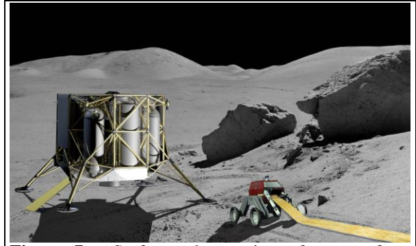
Figure 7. Surface teleoperation of rovers from orbiting facilities is a key technology for astronaut-assisted deployment of a lunar farside polyimide antenna and collection of geological samples. Image is courtesy of Robert MacDowell and NASA GSFC.
