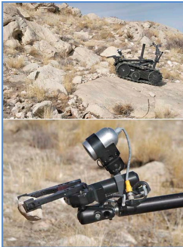
Fig. 1. (top) A Talon rover deployed at Meteor Crater, Arizona, for a field test of the human-assisted sample return concept. (bottom) A rock sample of impact ejecta recovered by the rover.
