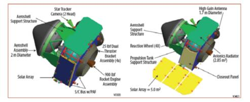
Artist's Concept of the VCM Carrier Spacecraft with solar array stowed and deployed.
