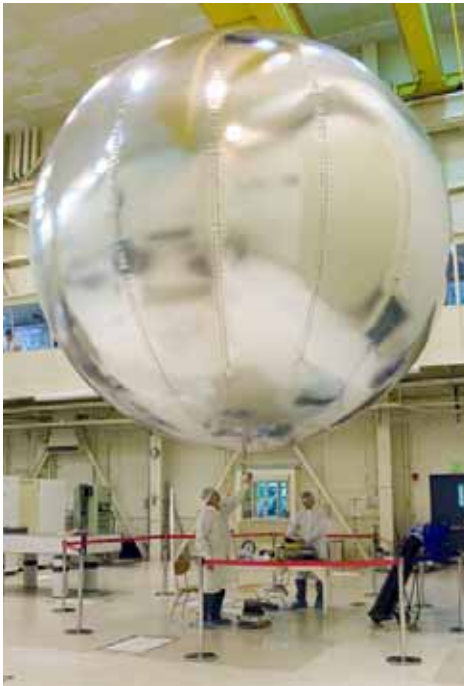
Fig 5-3: The most mature aerial platform concept is the super-pressure balloon concept (left). Solar powered conceptual airplanes (right) have been proposed for controlled flight on the day-side of Venus.
