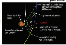
Note: At zenith the carrier S/C is directly overhead of the lander.
