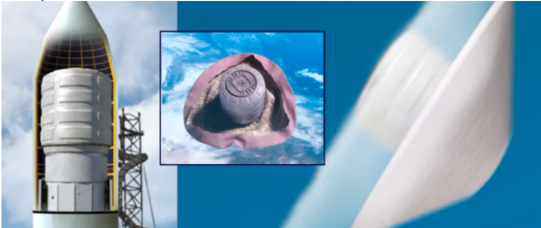
Hypersonic Inflatable Aerodynamic Decelerator (HIAD, LaRC)
